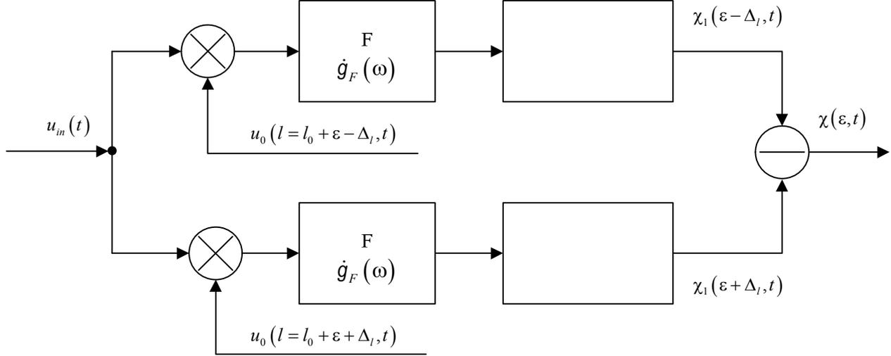
Fig. 2. Functional diagram of a two-channel discriminator with channels mismatched by the parameter  $l$
