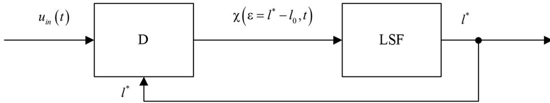
Fig. 1. Generalized block diagram of a tracking measuring device
