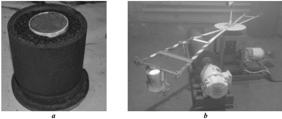
**Figure 1.** Appearance of the mold before combustion (a) and a multipurpose experimental centrifugal SHS installation (b).
