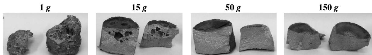
**Figure 3.** Appearance of transverse-cleft samples produced at various g values.
