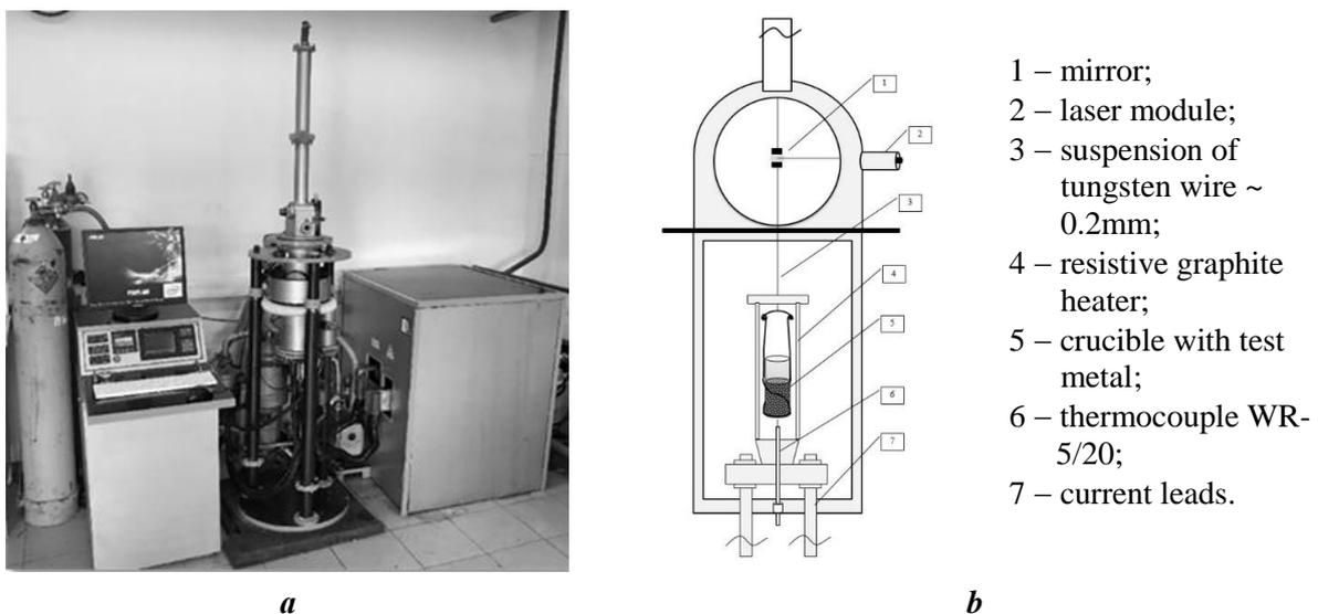
**Figure 2.** General schematic of the high-temperature system (a) and the overhead system (b) for measuring the viscosity of metal melts (HTV).
