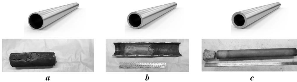
**Figure 5.** Experimental crystallizers of different wall thickness. (a) 3 mm, (b) 5 mm, (c) 6 mm.
