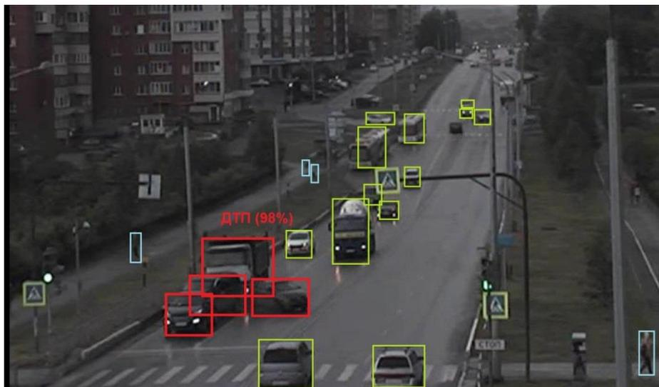
Fig. 4. An example of an accident detector by a traffic control video camera
