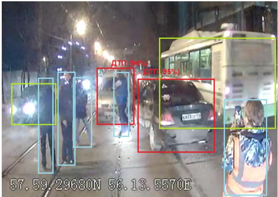
Fig. 3. An example of an accident detector on board of the passenger bus
