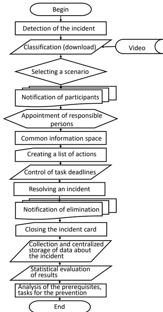
**Fig. 2.** Algorithm of the main functional steps for responding to an incident subject to the implementation of a full-cycle incident management system
